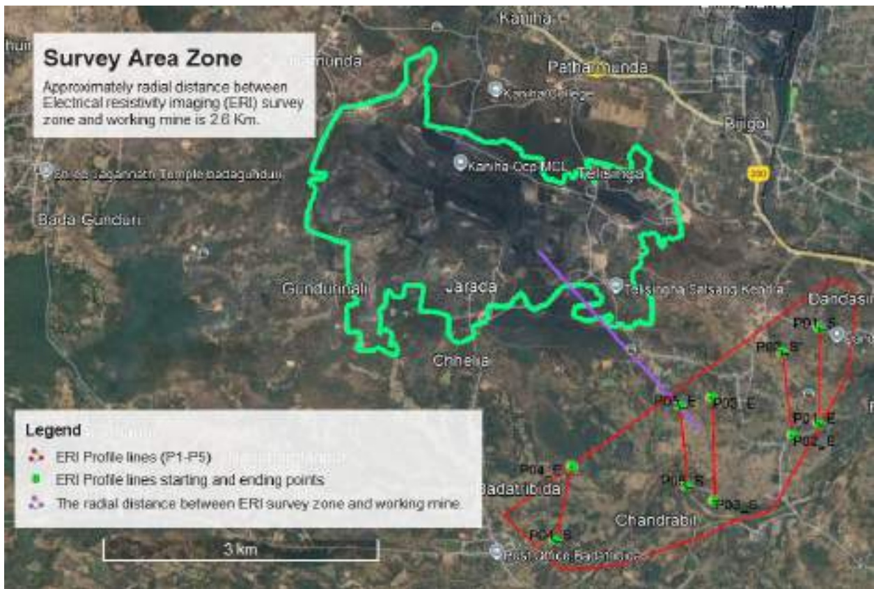
Figure.3.2.1: The Electrical resistivity imaging (ERI) survey Location, near Kaniha OCP mines.
